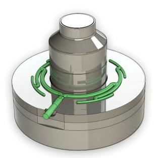
The spiral distribution zone, located between the second and third plates, is incorporated to provide better mixing, thermal uniformity and polymer distribution. The polymer flows across the spiral distribution zone toward the central pin. When the polymer reaches the central pin, it runs 90 degrees upward to the next layer or die lip. The central pin has internal heaters to aid in start-up and maintain process control.
