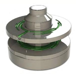
The flow splitting channels direct the polymer from the die entry location to each flow splitter. The flow splitting is performed in such a manner that the length of the channel is the exact same for each individual splitter. The die uses round cross-section flow splitting passages up to the spiral distribution zone to prevent dead zones and hang-up locations.
