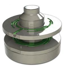
The flow splitting channels direct the polymer from the die entry location to each spiral. The flow splitting is performed in such a manner that the length of the channel is the exact same for each individual spiral. The die uses round cross-section flow splitting passages up to the spiral distribution zone to prevent dead zones and hang-up locations.
