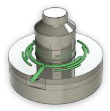
The spiral distribution zone, located between the second and third plates, is incorporated to provide better mixing, thermal uniformity and polymer distribution. The polymer flows across the spiral distribution zone toward the central pin. When the polymer reaches the central pin it turns 90 degrees upward to the next layer or die lip. The central pin has internal heaters to aid in start-up and maintain process control.
